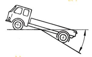
**4.8.3.4 Ground clearance between the axles:** means the shortest distance between the ground plane and the lowest fixed point of the vehicle.
