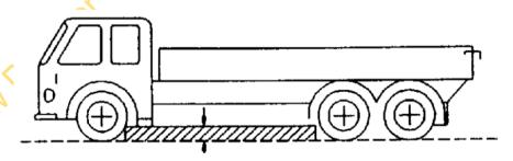
**4.8.3.5 Ground clearance beneath one axle:** means the distance beneath the highest point of the arc of a circle passing through the centre of the tyre footprint of the wheels on one axle (the inner wheels in the case of twin tyres) and touching the lowest fixed point of the vehicle between the wheels.
